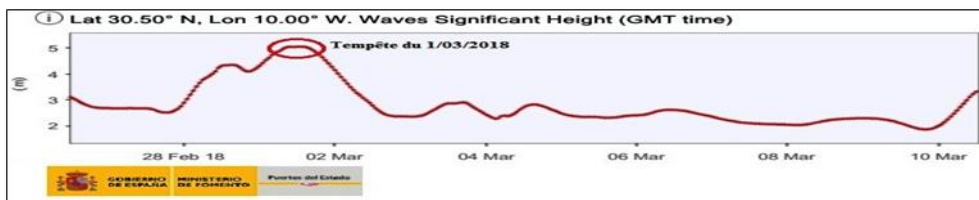
Fig.3: the significant wave height and its period at the time of the storm of 01/03/2018
